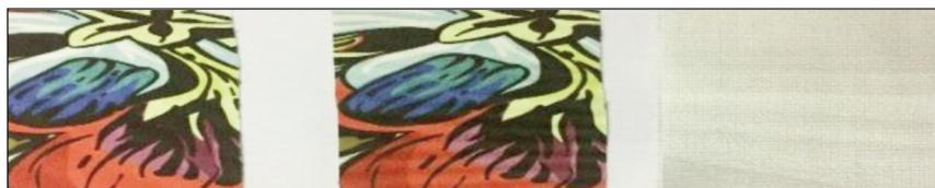
Fig. 14. Dry cleaning results for digitally printed samples
