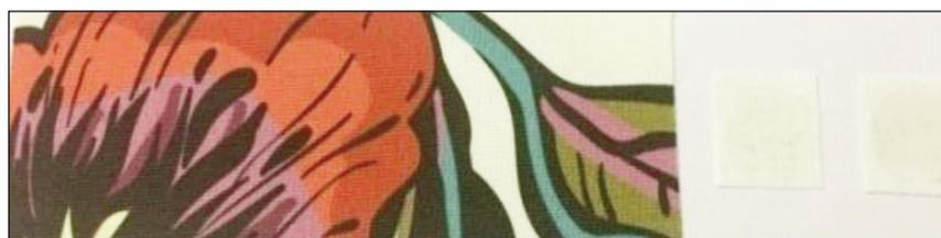
Fig. 11. Rubbing fastness of digitally printed fabric
